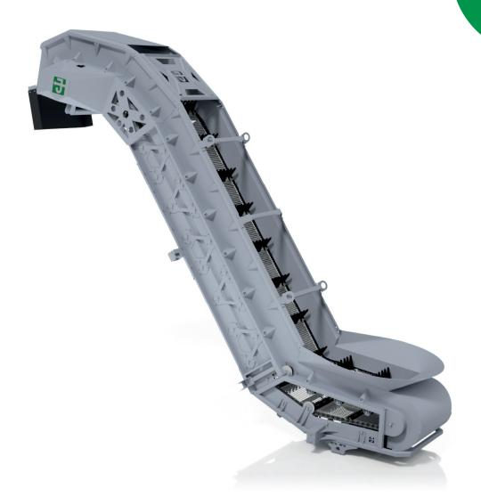
For years, traditional sugar cane elevators have required high maintenance. Broekema introduces a game-changing design: a low-maintenance elevator with improved cleaning functionalities. Broekema's innovative system uses a sieving web, carrying the cane up the incline, instead of scraping cane across the elevator floor. This patented design, with its larger sieving area, also removes more debris, leading to a cleaner harvest and a reduced cost of ownership per acre.
